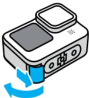
2. With your camera off and battery removed, insert the SD card into the card slot with the label facing the battery compartment.
