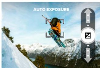
Slide up to brighten the image. Slide down to darken it. You can adjust up to 2 stops in either direction.
